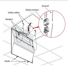
The panel hangers are inserted into the notches on the mounting rail, enabling the panel to hang freely while electrical connections are completed.
