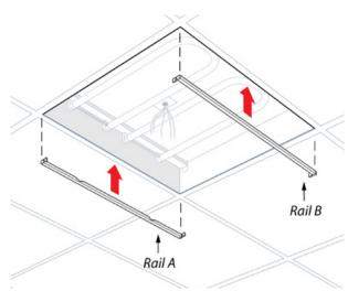
The mounting rails are inserted between the troffer and grid rail on oppositie sides with the anti-rotational tabs pointed inward and notches facing up.
