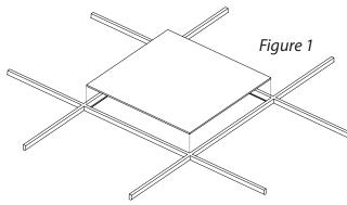
**4.** Raise the protective lens into the empty grid space, then lower until it lies on the T-grid bar properly. Then move the light panel to the right top of the protective lens until the light panel rests on the same T-grid bar properly (Figure 3).
