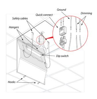
The panel hangers are inserted into the notches on the mounting rail, enabling the panel to hang freely while electrical connections are completed.
