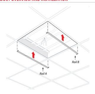
The mounting rails are inserted between the troffer and grid rail on opposite sides with the anti-rotational tabs pointed inward and notches facing up.
