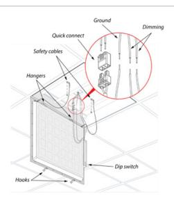
The panel hangers are inserted into the notches on the mounting rail, enabling the panel to hang freely while electrical connections are completed.
