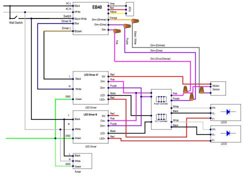
Note: \* LED Driver A near the power/CCT controller should be connected to
