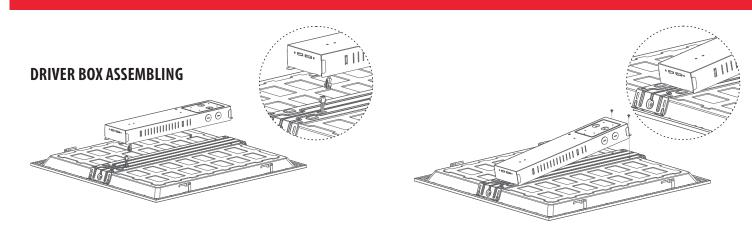
**1.**Connect the driver to the panel with quick plug connector.
