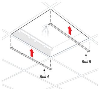
The mounting rails are inserted between the troffer and grid rail on oppositie sides with the anti-rotational tabs pointed inward and notches facing up.
