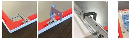
Integrated Grid Clips bend up and out. Then, when lowered into the ceiling, they catch on T-grid bar, for added support.
