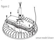
Close and secure the new plate to the fixture. Ensure gasket is in place to guarantee seal is water proof.
