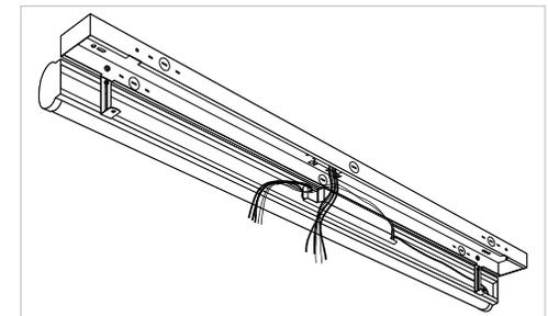
6. Swing the hanging lamp into final position. Ensure that the hanging brackets are flush to the outside of the housing wall. Put screws in to secure brackets to housing.
