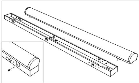
3. Locate the surface mounting holes. Raise empty fixture into place and drive two mounting screws (not provided) directly into the mounting surface/anchors.
