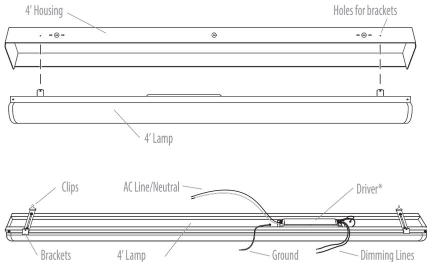
\* Driver equipped with magnets for easy attachment.
